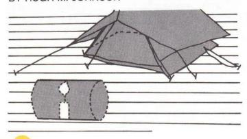
his little radiant heat stove will keep your tent warm, or your duck blind from turning into an icebox. You need a #10 can with both ends cut out and a thick candle about 3" long. Tear all the paper from the can, flatten one side so it won't roll around. Let a few drops of wax melt from the candle onto the inside of the can at the center to form a puddle to set the candle in. The wax will cool and hold the
